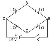
29. In the circuit given find the current through each resistor.
